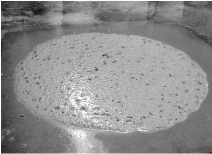
VSI 2: Unstable mix, visible separation around edges (halo) and bleeding.
