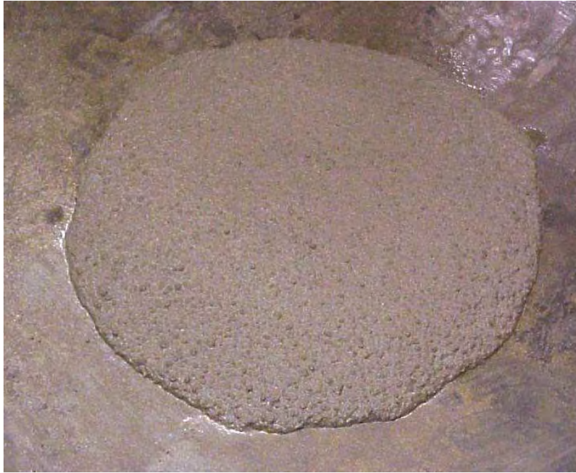
VSI 0: Stable mix, no evidence of segregation or bleeding.
